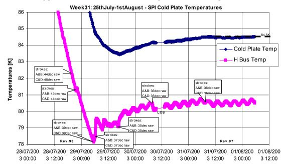
The following plot shows the current and the temperature parameters of the cryocooler during the active cooling: current, power, temperatures and phase were all nominal.
