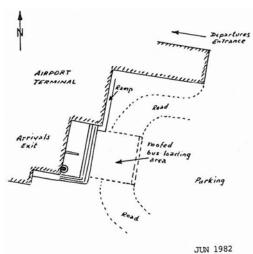
The station is located in front of the 4 doors to the S of the main exit of the arrivals terminal—It is on the concrete surface of the top step, 40cm S of the door and 10cm E of the wall. Although no BM was found in 1968, this station is believed to coincide exactly in elevation and very nearly in location with the original "K" site. In 1982 a 2cm square plug was found at the site which has become the monument for the station.
