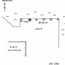
The station is located on the concrete platform of the 2nd bollard, 11.5m E of the NW corner of the cock. The station is monumented with a Geodaetisk Institut bronze plug.
