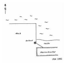
The station is located on a concrete platform for a bollard at the SE end of the dock by the havnekontor. It is monumented with an aluminum disc.
