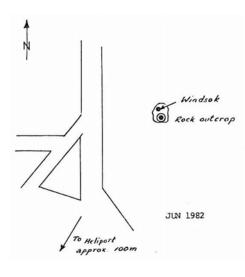
The station is located on a rock outcrop 2m S of the windsok, NE of the heliport. It is at the site of a survey point identified by a white painted circle with a black ring around it. The survey point is GTO 55864.
